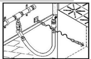
**AWARNING**: Per ANSI Z223.1 & ANSI Z21.69, the restraining cable must remain installed and connected while the flexible gas connector is installed.
